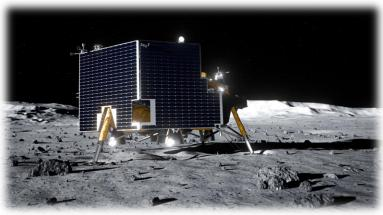
Astrobotic will demonstrate long-distance (500m), high power (1 kW @ 1kV, 1khZ, 1¢ AC) transmission on the Moon by maturing and delivering a technology demonstration payload, named LunaGrid-Lite (LGL)
